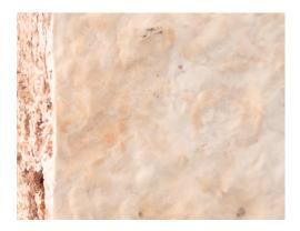
**MykoFoam** is an acoustic and thermal carbon-negative insulation sheet. It is 100% made of renewable and biobased materials sourced from industrial waste. Our technology presents improved water-proofing and stabilising properties for increased durability, whilst maintaining the breathable and fire-retardant benefits of mycelium insulation.
