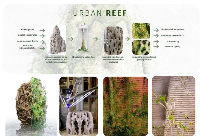
**3D printing** with ceramics in order to create habitats that stimulate spontanous ecologies. For this Urban Reef works with a range of different material mixtures and integrated biofilms for biorecepticity.
